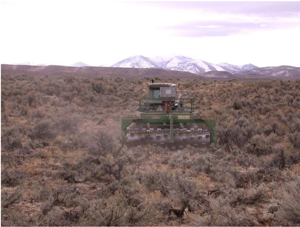
Photo 5: Aerator working under dry conditions.
