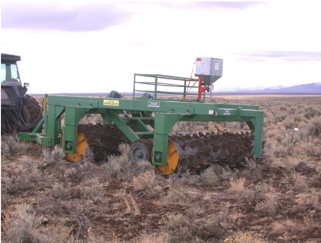
Photo 4: Aerator in operation – second strip.
